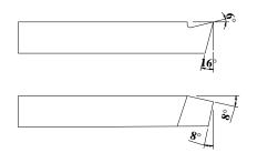
10. Make plain surfaces (four surfaces) using surface Grinder
