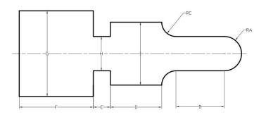
2. Using Stock removal cycle – Create a part program for multiple turning operations and produce component in the Machine.
